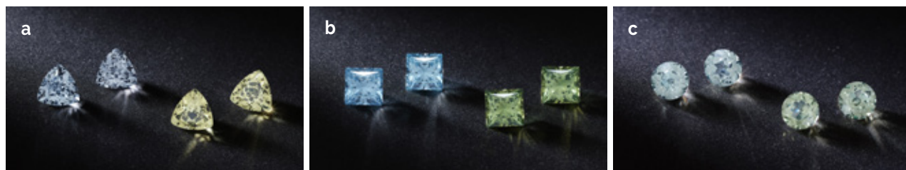
Figure 34: Representative synthetic sapphires from a parcel recently examined by the authors show the changes in colour before (left side) and after (right side) exposure to short-wave UV: (a) pale violetish blue to yellow (6 × 6 mm), (b) moderate blue to greenish yellow (5 × 5 mm) and (c) pale bluish green to greenish yellow (5 mm in diameter). Composite photos by Daniel Maldonado, Stuller Inc.
